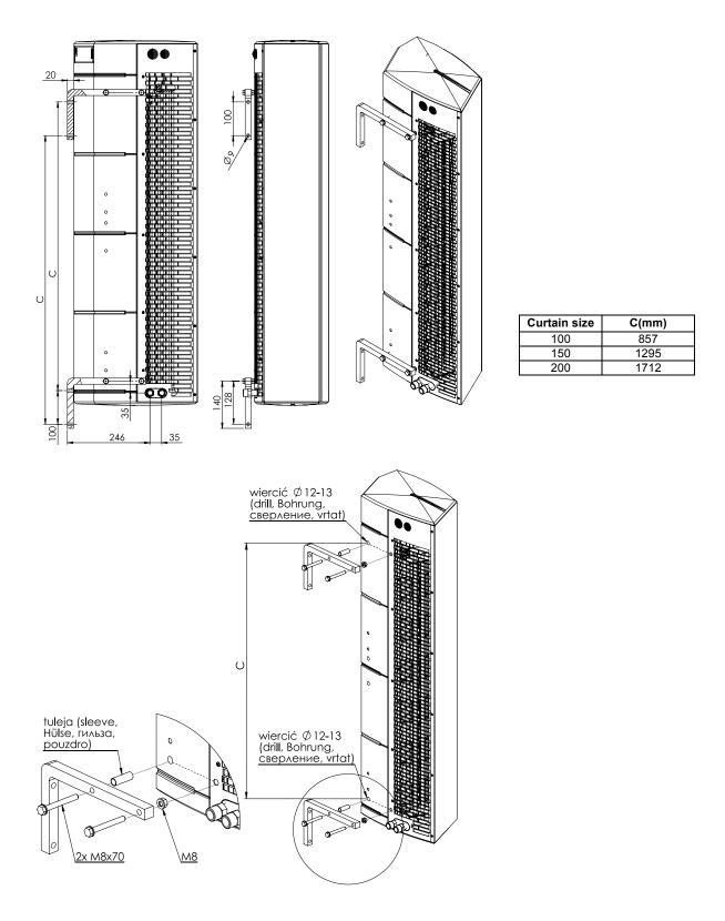
It is important to note that the minimum distance between the unit and the floor for installation with engine at the bottom is not less than 100mm. This allows access to the electrical terminal strip and to the water exchanger vent.
